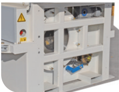
Protected drive unit with labyrinth seal
