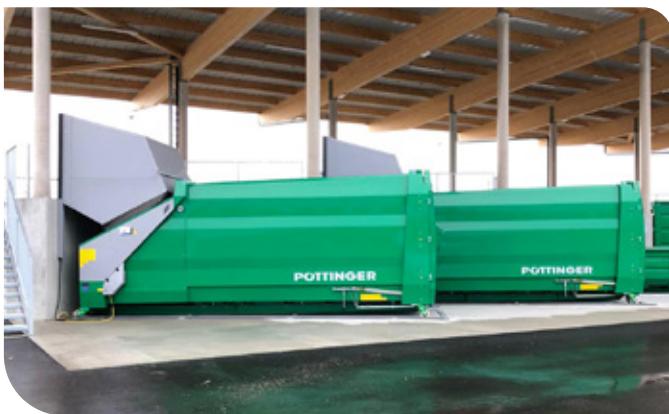
Sluice for plastic packaging with insertion slot and access system
