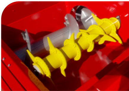
Standard screw conveyor and intake system with own drive unit
