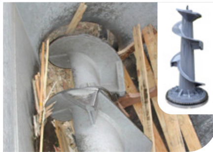
Wood screw conveyor for efficient processing of wood waste, such as whole europallets
